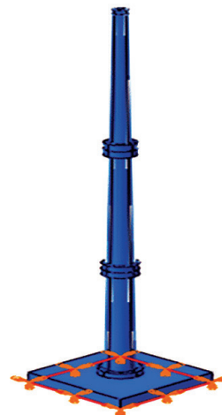
Figure 5. Applying boundary condition for UHPFRC communication tower
